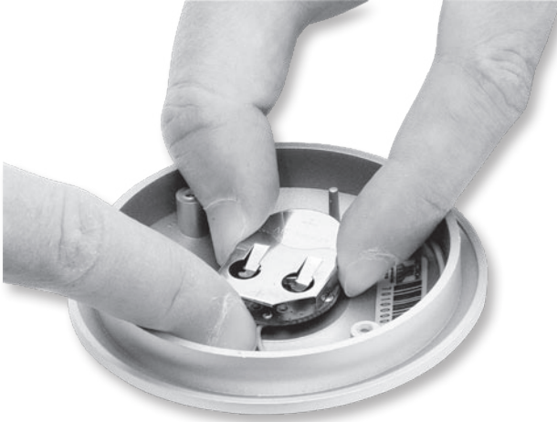
Fig. 10: inserting the new battery
