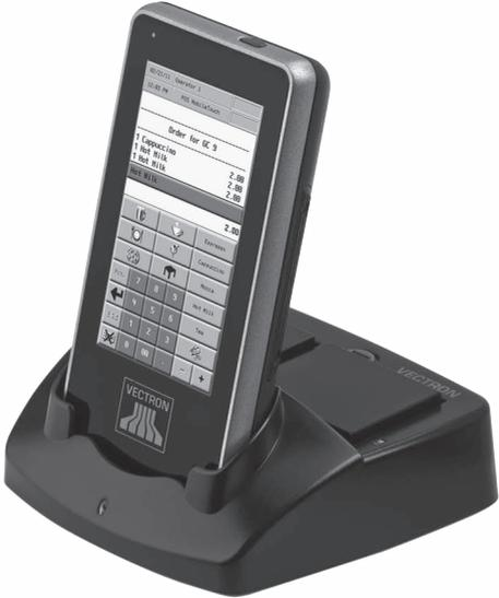
Fig. 34: Vectron POS MobileTouch
