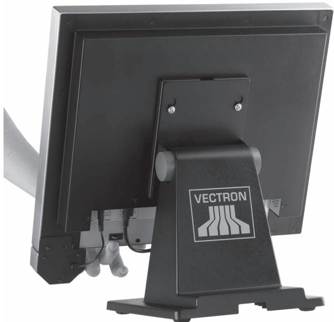
Fig. 17: Switching off the SteelTouch II
