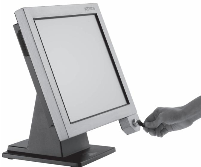
Fig. 14: Approaching the key to the operator lock
