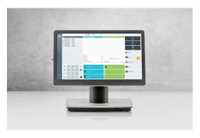
Münster, 10 August 2020 – With POS 7, the Vectron Systems AG will launch a modular high-end POS system with intuitive layout, swipe function and 15,6" Full HD display in September. It consists of a system box, holder and display unit. Due to the new modular concept, the hardware can be flexibly adapted. The system box made of high-quality metal can be easily separated from the rest of the hardware and can thus be mounted under the counter, for example. This
